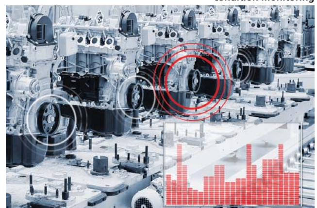
1 In-line acoustic condition monitoring
