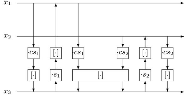
Figure 4: Combined rounding in two succeeding lifting steps
