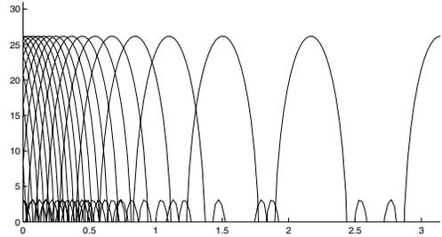
Fig. 3. WDFT-filterbank with  $N = 32$ ,  $\lambda = -0.6865$
