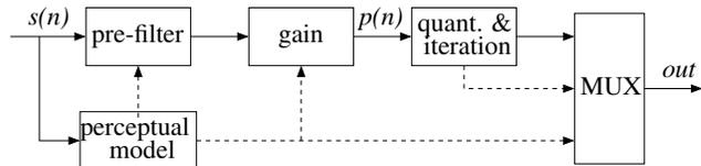
Fig. 1. Basic structure of our ULD Encoder
