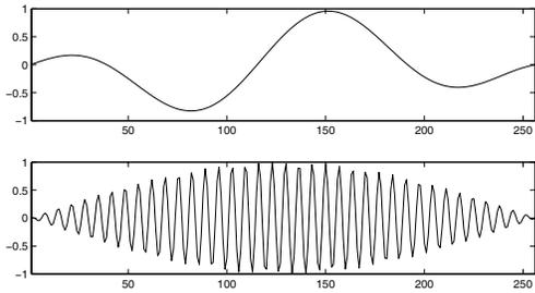
Fig. 6. WDFT-filter bank,  $N = 256$ ,  $\lambda = -0.6865$ , impulse response of 10th band (upper) and 100th band (lower)
