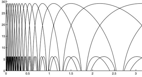
Fig. 5. WDLDFT-filter bank with  $N = 32$ ,  $\lambda = -0.6865$
