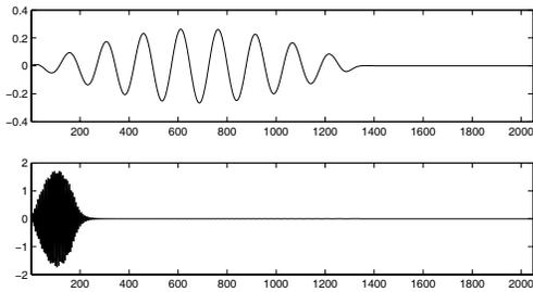
Fig. 7. WDLDFT-filter bank,  $N = 256$ ,  $\lambda = -0.6865$ , impulse response of 10th band (upper) and 100th band (lower)
