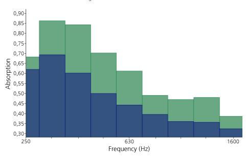
Transmission loss measurement of an acoustic panel (perforated sheet with mineral wool) with and without synthetic fibre covering
